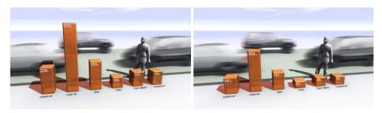
Actual volume of greenhouse gas emissions per passenger mile (left) or per passenger kilometre (right) for different forms of transport, expressed in terms of  $CO_2(e)$  – carbon dioxide equivalent. (Figures for cars relate to the driver only.)
